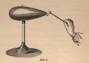
On an insulated cylinder, with the two hemispheres at the ends, the density of the electricity is greatest at the ends. On a circular disk, the density is greatest at the edges. The tendency is for electricity to accumulate at points. On a sphere the density is uniform; the further removed a body is from a sphere the more irregular the distribution.
